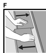
**F) Disassemble the panels by sliding the short ends horizontally or fold up a panel.**
