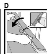
**C) Remove the vertical locking part of the strip with a chisel.**
