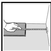
**5) At the end of the first row,** put a spacer to the wall allowing for 5/16" (8mm) expansion and measure the length of the last plank to fit.
